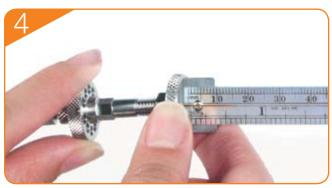
Hand-tighten the column nut into the gauge until the ferrule starts to compress. Adjust the length of the column to the desired length. Further tighten the nut into the gauge until the column cannot slide.
