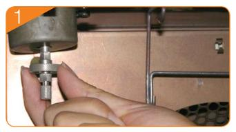
Detach the Cool-Lock Nut and column from GC instrument.
