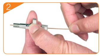
Insert column through column nut and ferrule. Cleanly  $cut \ge 1$  cm of the column that is protruding from the nut and ferrule.
