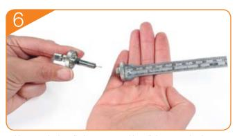
Unscrew the installation gauge and install the nut and column into the instrument. Make sure Cool-Lock nut is in the full extension position to achieve the correct premeasured position, and allow for proper leak checking.
