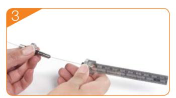
Insert the end of the column and column nut into the bottom of the Cool-Lock Nut Installation Gauge.
