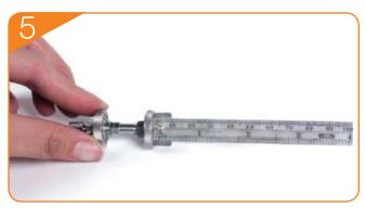
Tighten its bottom ferrule. Make sure lower body/ ferrule is in the full extension position.
