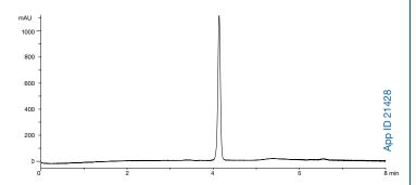
Column: Gemini 3 µm C18 Dimensions: 150 x 4.6 mm Part No.: 00F-4439-E0
