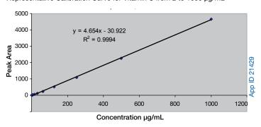
Table 1. Calibration Curve from a Gemini® 3 µm C18 Column Based on ChromaDex® Reference Materials
