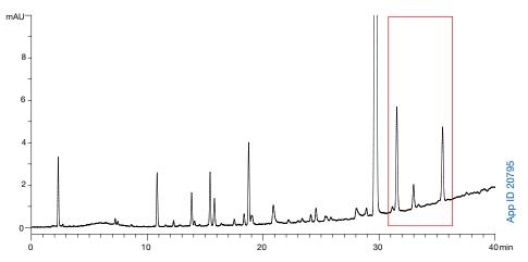
b. Phenomenex Kinetex<sup>®</sup> 5 µm C18 250 x 4.6 mm; Backpressure = 188 Bar
