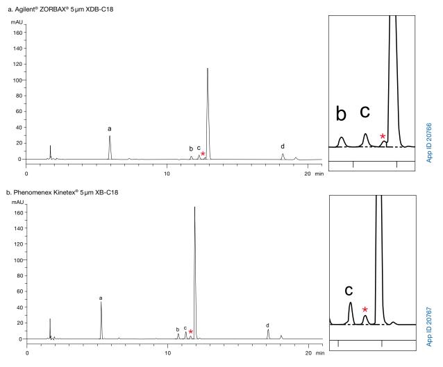
Conditons for both columns Column: Kinetex 5 µm C18 ZORBAX 5 µm XDB-C18 Dimensions: 250 x 4.6 mm Mobile Phase: A: TFA/Water/THF (5/900/100) B: TFA/Acetonitrile/THF (5/900/100 Time (min) % B 0 10 % Gradient: Time (min) 40 80 % Flow Rate: 1.5 mL/min Temperature: 40 °C Detection: UV @ 295 nm 4. Unidentified Sample: 1. Impurity A 2. Impurity B 3. Impurity C 5. Paroxetine 6. Impurity D
