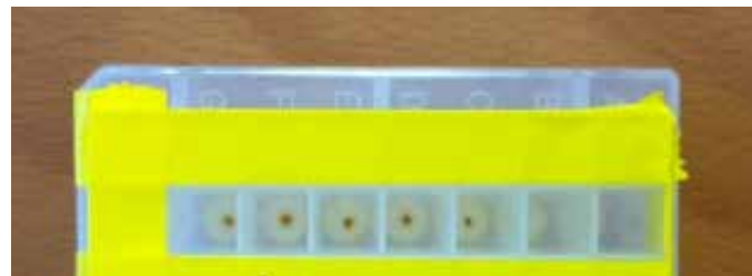
Trapped-precipitated-enzyme on Impact following enzymatic hydrolysis using acetonitrile
