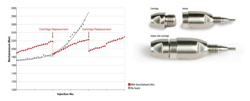
Accelerated lifetime test using endogenous biological matrix on Kinetex 2.6  $\mu$ m C18 50 x 4.6 mm ID
