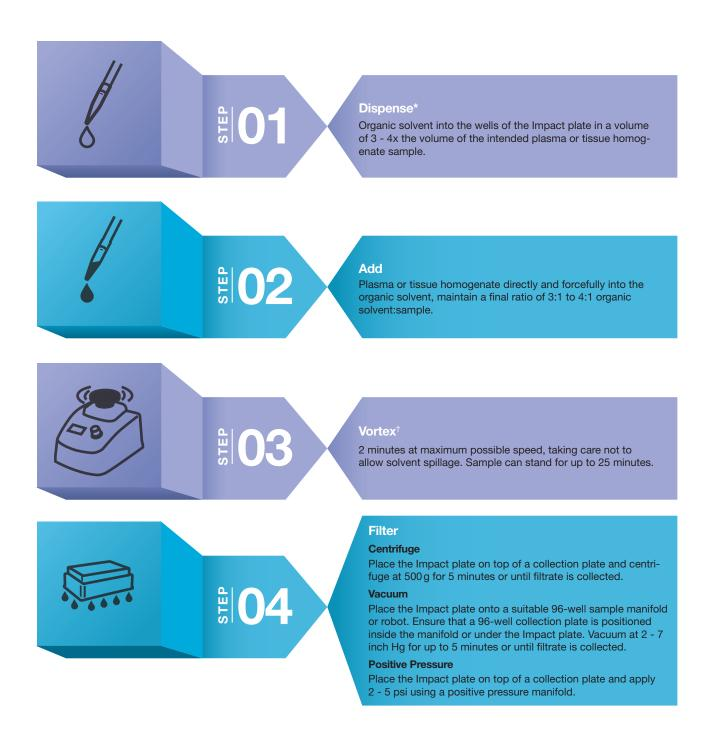
\* A 3:1 v/v ratio of organic solvent to biological sample will dilute your sample less. In contrast, a 4:1 v/v ratio of organic solvent to biological sample will ensure a more complete precipitation. A 4:1 v/v ratio is recommended when using methanol.
