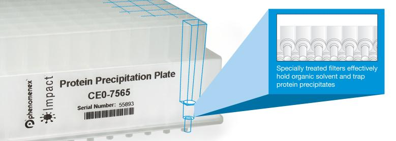
Impact protein precipitation plates with Solvent Shielding Technology<sup>™</sup> offer a rapid and convenient way to remove proteins from plasma and tissue samples prior to analysis. The Solvent Shielding Technology design will withold organic solvents above the filter membranes for up to 25 minutes, allowing for direct in-well precipitation upon sample addition. The precipitate is then filtered out via vacuum, centrifuge or positive pressure resulting in a clean, protein depleted extract.
