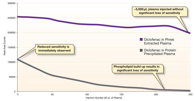
To assess the effect of phospholipid build up, repetitive 20 µL injections of diclofenac in protein precipitated plasma versus diclofenac in Phree extracted plasma were made.
